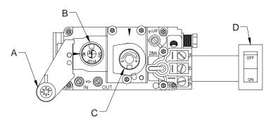
NOTE: Knob cannot be turned from "PILOT" to "OFF" unless knob is pushed in slightly. Do not force.
